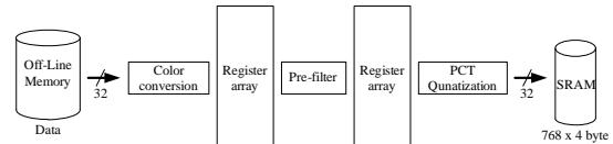
Fig. 15. Data flow of JPEG XR stage 1.
