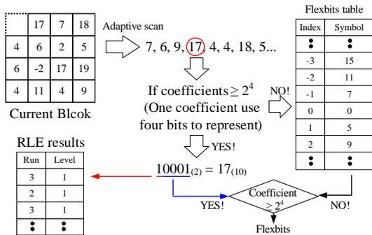
Fig. 13. Adaptive scan and Run-Level encode example – AD, and AC.
