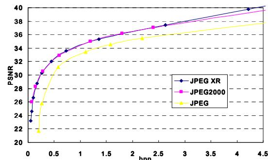
Fig. 6. PSNR Comparison between different image standard.
