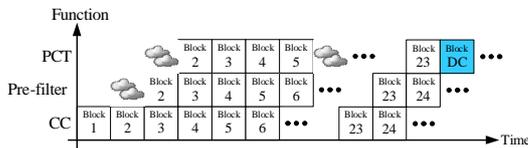
Fig. 17. DC block insertion on the function block pipeline.
