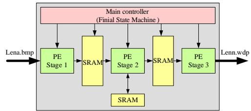
Fig. 14. Pipeline stage consideration of JPEG XR.
