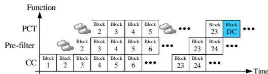
Fig. 17. DC block insertion on the function block pipeline.
