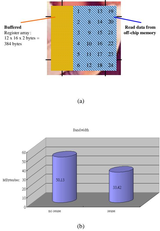
Fig. 16. Data reuse of pre-filter and PCT function.
