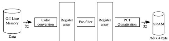
Fig. 15. Data flow of JPEG XR stage 1.
