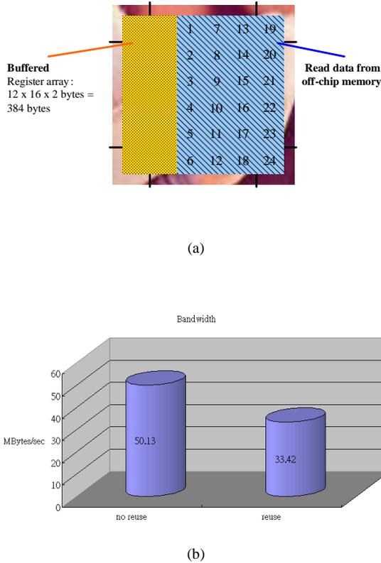
Fig. 16. Data reuse of pre-filter and PCT function.
