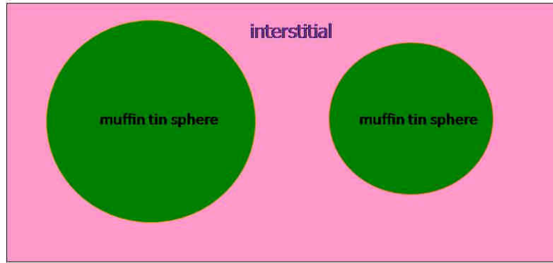
Figure 6: A unit cell is divided into the muffin tin spheres and the interstitial region when the APW basis is used.
