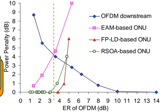
Fig. 7. Power penalties of downstream OFDM and upstream NRZ signals generated by different kinds of ONUs against different extinction ratio (ER) of the downstream OFDM signal.
