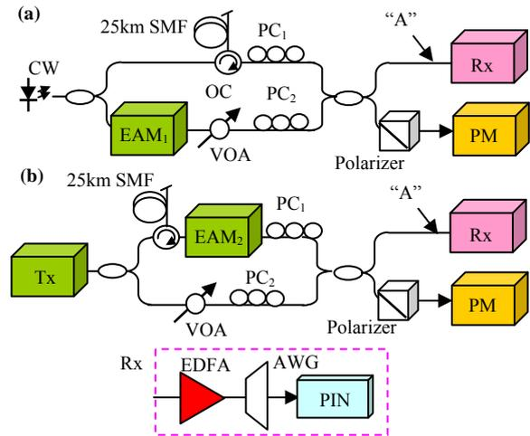
Fig. 2. Experimental setup to emulate (a) Carrier-RB and (b) Signal-RB. EAM: electro-absorption modulator, VOA: variable optical attenuator, PC: polarization controller, PM: power meter. Inset: Rx architecture, AWG: arrayed waveguide grating.
