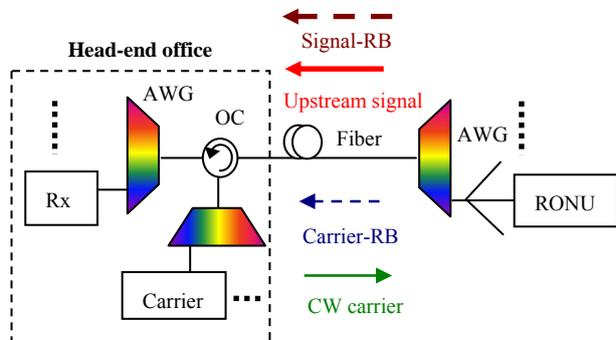
Fig. 1. Schematic of WDM PON using centralized light source. AWG: arrayed waveguide grating, OC: optical circulator, Rx: receiver, Carrier-RB and Signal-RB: carrier and signal generated Rayleigh backscattering.
