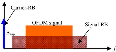
Fig. 4. Schematic RF spectra indicating the carrier-RB, signal-RB of OFDM signal.
