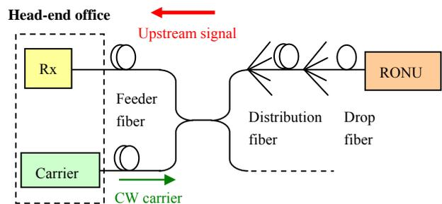
Fig. 5. Schematic of a carrier distributed PON using dual-feeder fiber architecture.
