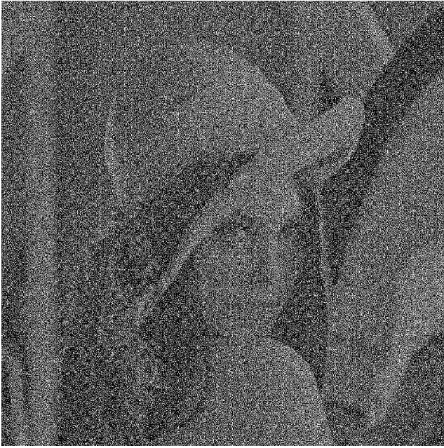
Fig. 6. Stacking “any” two transparencies (e.g. 1st and 3rd transparencies here) yields an enlarged binary image of Lena.
