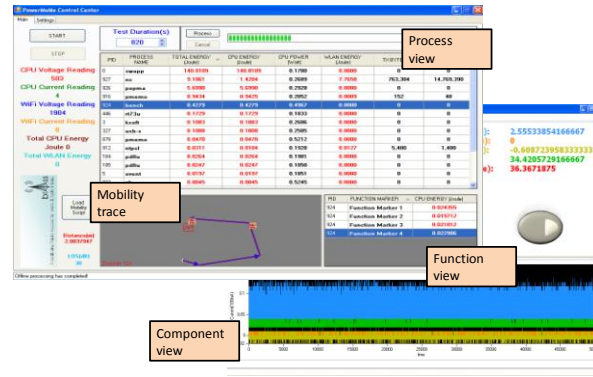
Figure 8. The GUIs displaying energy profiling results for each process, function, and mobile mobility path.
