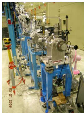
Figure 1. (a) Experimental Chamber for Researches of EUV Detector and Radiation Damage. (b) Measured and simulated response of the MOS tunneling photodetector with the Ag gate electrode.
