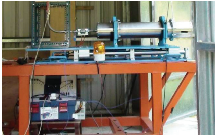
Figure 4 Previous hybrid combustion chamber (left) and mounted on the test stand
