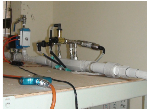
Figure 24 The venturi flow meter with pressure transducers used in the experiments.
