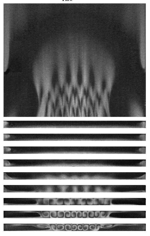
Fig. 1 Top and end view flow photos at steady state for Re=25, Ra=9,200 at y=1/2 and (a)z=0.1, (b)z=0.2, (c)z=0.3, (d)z=0.4, (e)z=0.5, (f)z=0.6, (g)z=0.7, (h)z=0.8 and (i)z=0.9.
