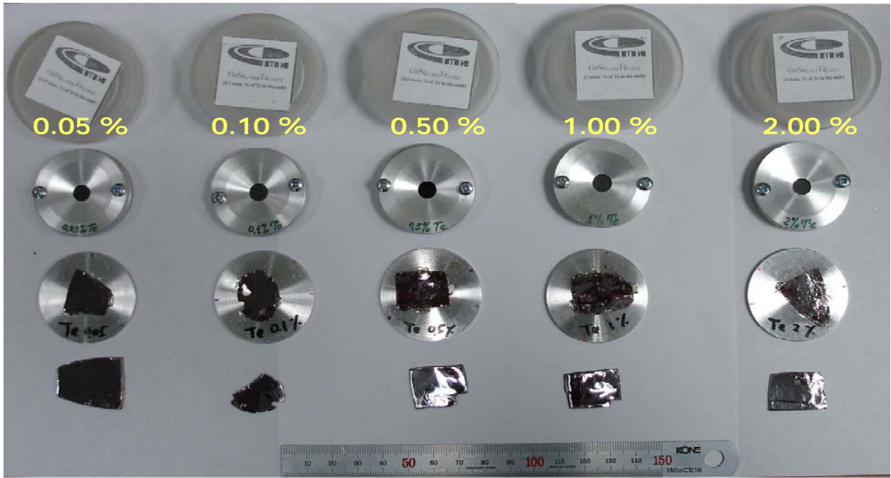
Fig. 3-2 External view of the GaSe:Te samples with 0.05, 0.10, 0.50, 1.00, 2.00 mass%.
