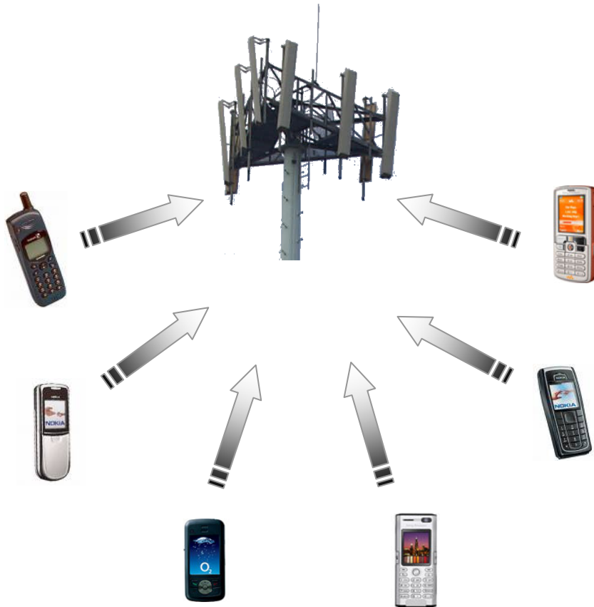
Fig. 1.1 Schematic diagram of uplink transmission.
