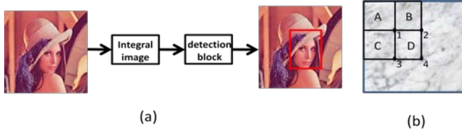
Figure 1 (a) Viola-Jones face detection procedure (b) Integral image computation.
