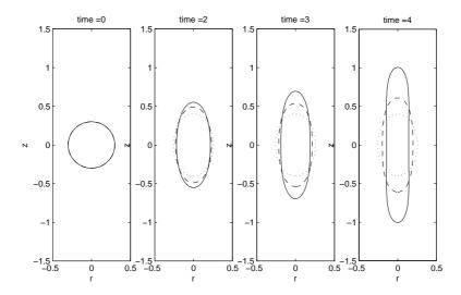
FIGURE 1. The time evolution of a drop in an extensional flow with different capillary numbers. Three different plots are as follows: (1) clean interface with Ca = 0.3: dotted line '..'; (2) clean interface with Ca = 0.4: dashed line '-'; (3) contaminated interface with Ca = 0.3: solid line '-'.
