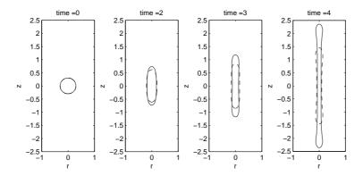
FIGURE 3. The time evolution of a drop in an extensional flow with different equations of state. Here,  $Pe_s = 180$  and Ca = 0.5. (1) linear EOS: dashed line '-'; (2) nonlinear EOS: solid line '-'.
