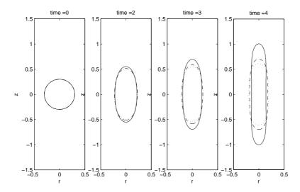
FIGURE 2. The time evolution of a drop in an extensional flow with different surface Peclet numbers. Three different numbers are used: (1)  $Pe_s = 1.8$ : dotted line '..'; (2)  $Pe_s = 18$ : dashed line '-'; (3)  $Pe_s = 180$ : solid line '-'.
