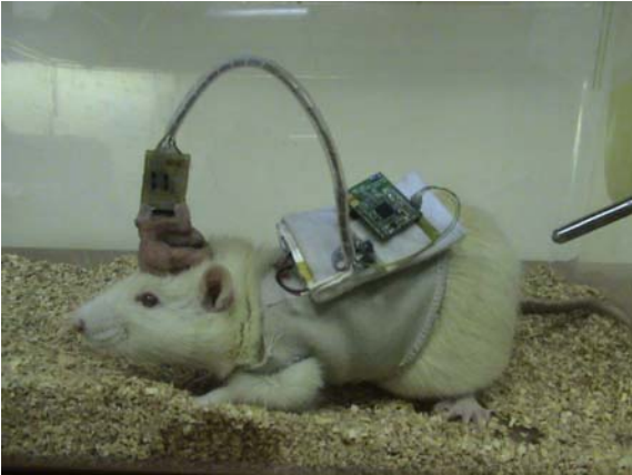
Fig. 14. The developed wireless multi-channel behavioral state monitoring system installed on a rat.
