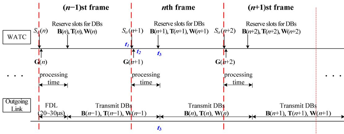
Fig. 4.3 Timing sequence in a node
