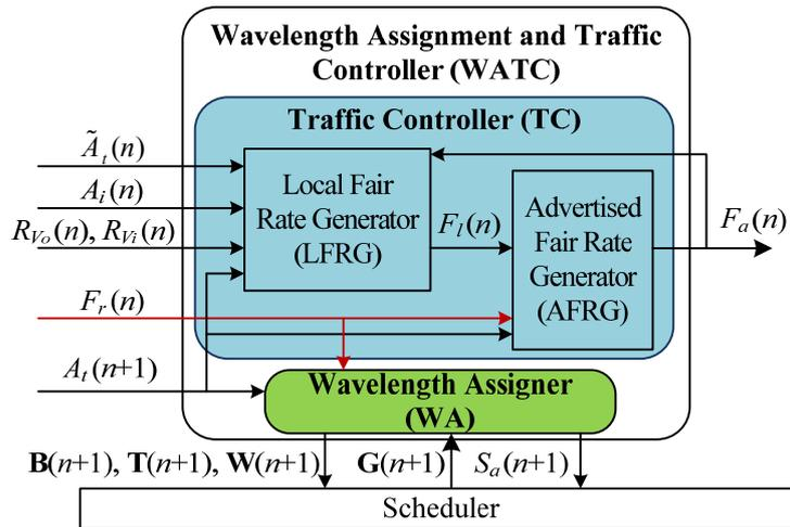
Fig. 4.4 The structure of WATC
