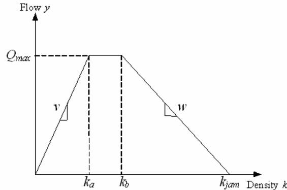
Figure 9. Fundamental diagram of CTM
