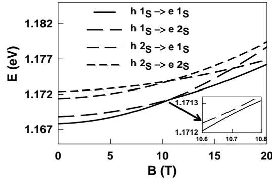
Figure 3. Lowest transition energies in the double dot molecule as functions of magnetic field  $B||z$ . Inset: the anticrossing region.
