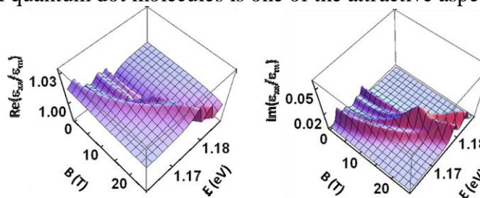
Figure 10. Effective permittivity of an array of embedded quantum dot molecules (distance between the dots in the quantum dot molecule is 10 nm,  $\mathbf{B}||z$ ): (a) real part and (b) imaginary part.
