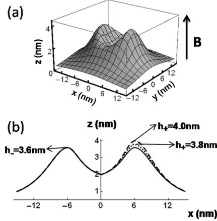
Figure 19. (a) Geometry of the asymmetrically wobbled InAs/GaAs nano-ring for  $\delta_h \approx 5.5\%$ . (b) Projection of the ring height onto the  $x$ - $z$  plane for:  $\delta_h = 0\%$  (solid curve);  $\delta_h \approx 5.5\%$  (dotted curve);  $\delta_h \approx 11\%$  (dashed curve).
