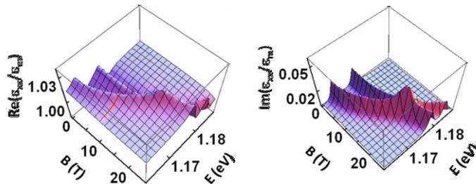
Figure 9. Effective permittivity of an array of embedded quantum dot molecules (distance between the dots in the quantum dot molecule is 20 nm,  $\mathbf{B}||z$ ): (a) real part and (b) imaginary part.
