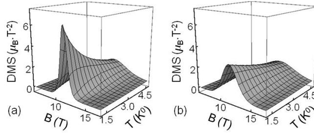
Figure 24. Dependence of the differential magnetic susceptibility (DMS) on magnetic field and temperature: (a) a single ring; (b) differential magnetic susceptibility averaged within an ensemble of the rings.
