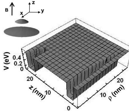
Figure 17. Mapped confinement potential of a double dot molecule
