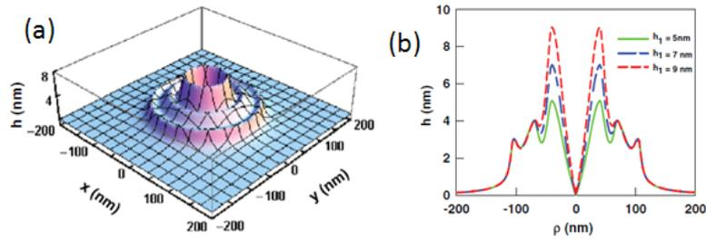
Figure 25. (a) Three-dimensional geometrical shape of a triple concentric nano-ring. (b) Two-dimensional geometry of triple concentric nano-rings with variation of the inner height.
