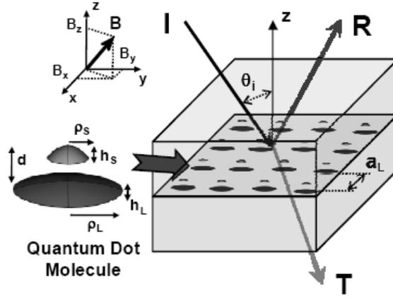
Figure 2. Schematic of the magneto-optics of a layer of embedded semiconductor quantum dot molecules.
