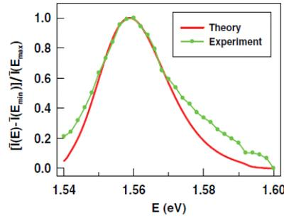
Figure 26. Normalized averaged intensity of the optical transitions of the ring ensemble as a function of the energy at low temperatures.  $E_{min}$  and  $E_{max}$  are the positions of the intensities' minimum and maximum.
