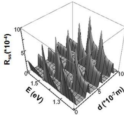
Figure 8. Reflectance of the quantum dot multilayered structure consisting of five layers as a function on the transition energy and distance between the consecutive layers.
