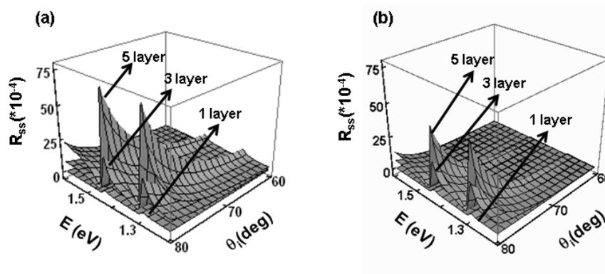
Figure 7. Reflectance of the quantum dot multilayered structures as a function on the transition energy and angle of incidence: (a)  $d = 10\text{nm}$  and (b)  $d = 50\text{nm}$ .
