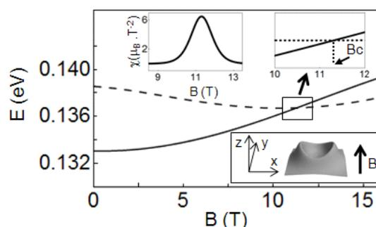
Figure 23. Energy states and differential magnetic susceptibility (upper left inset,  $\mu_B$  stands for the Bohr magneton) of a wobbled nano ring.
