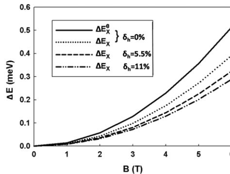
Figure 21. Diamagnetic shift of the ground state energy of the exciton confined in the ring for different wobbling asymmetries ( $\Delta E_X^0$  presents the optical transition energy diamagnetic shift for non-interacting electrons and holes).
