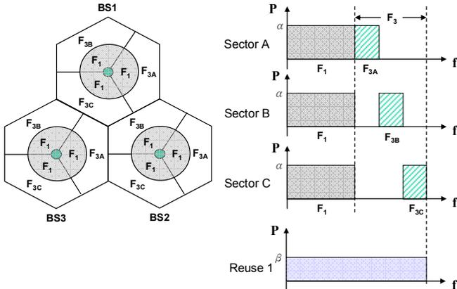
Figure 1. Spectrum setting for partial reuse in a tri-sector cell layout
