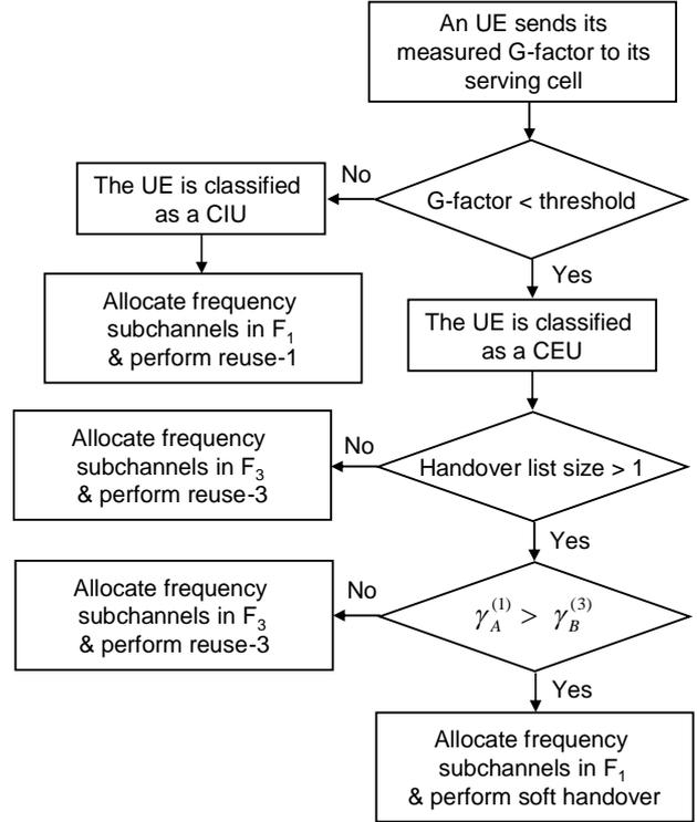
Fig. 2. Operational flow chart of the proposed hybrid scheme
