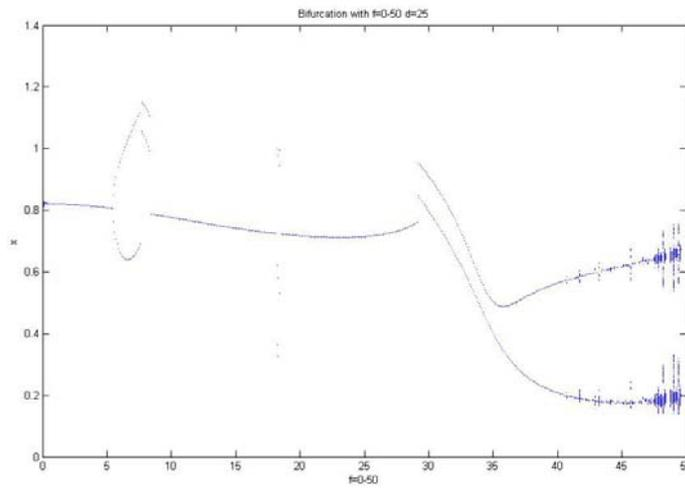
Fig. 2 Bifurcation diagram for autonomous new Mathieu-van der Pol system  $f=0\sim 50$ .
