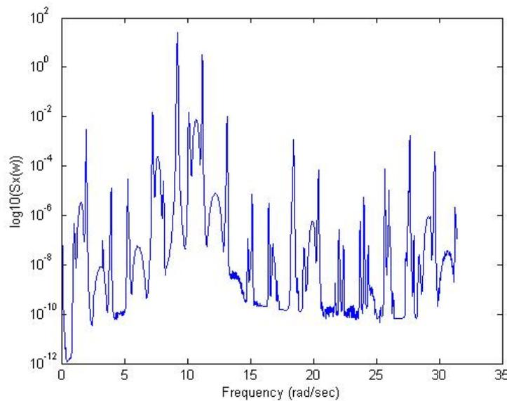
Fig. 4 Power spectrum for autonomous new Duffing-van der Pol system.
