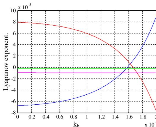
Fig. 3. Lyapunov exponents of controlled Quantum-CNN system.
