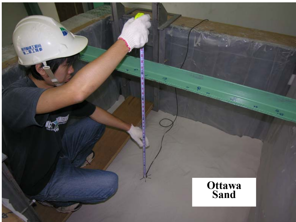
Fig. 14. Placement of SPT in Soil Mass
