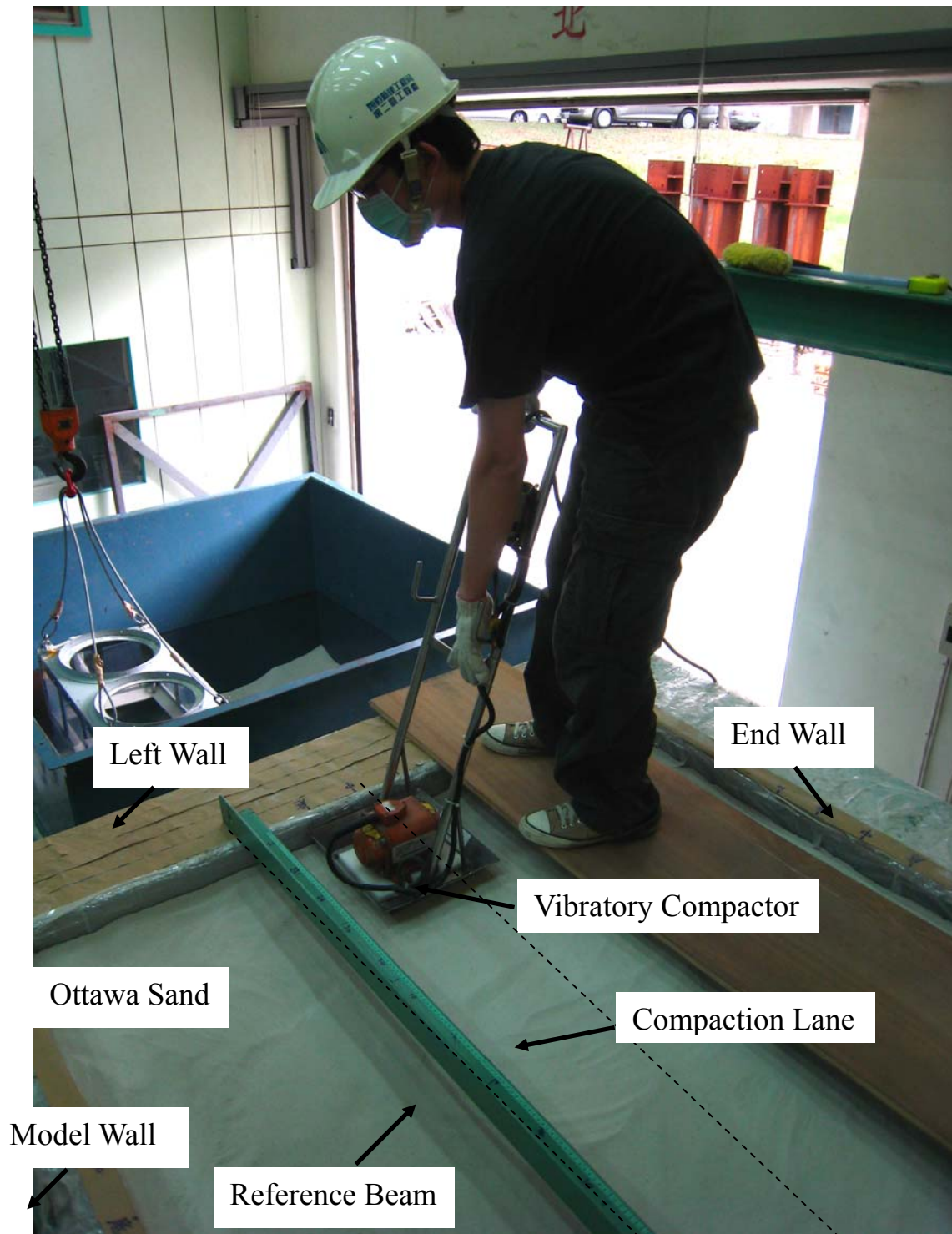
Fig. 21. Compaction on Surface of Backfill
