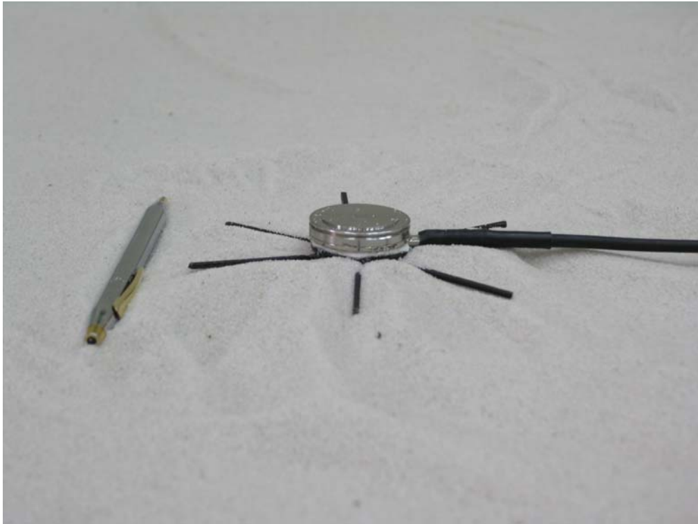
Fig. 15. SPT used to Measured Vertical Stress
