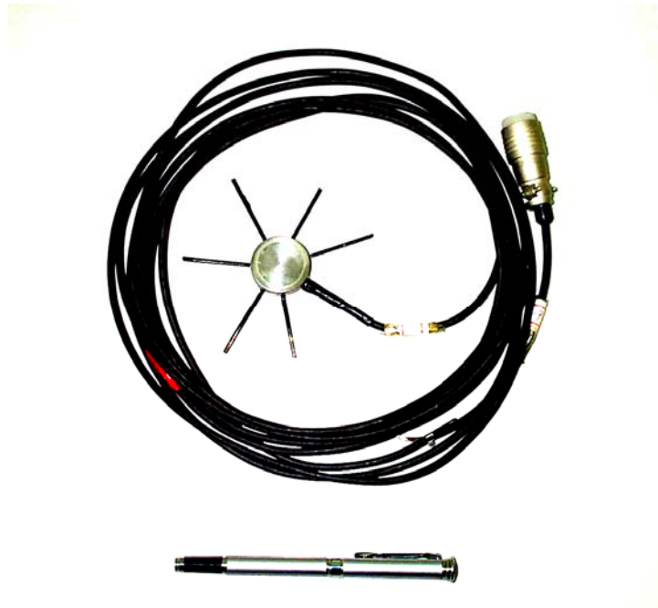
Fig. 7. Soil-Pressure Transducer (Kyowa BE-2KCM17) (after Chen, 2002)
