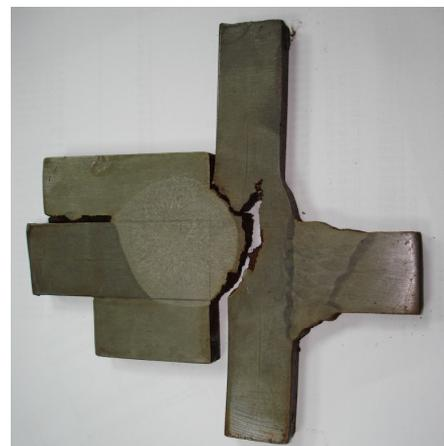
Fig. 3 Failure at the electro-slag welding
