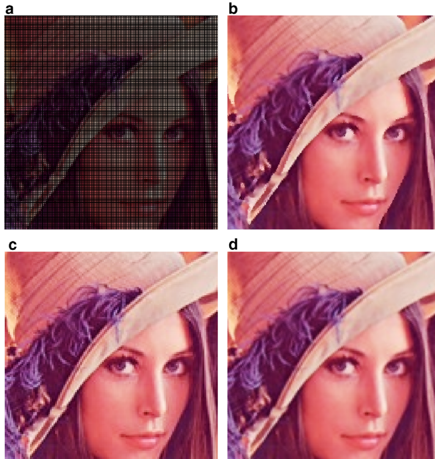
Fig. 12. Comparison of results of different interpolation methods for image expansion. (a) Raw enlarged image. (b) Result of proposed method. (c) Result of simple pixel duplication. (d) Result of 4NN interpolation method. Note that the original image size is 256 \times 256 ; which is enlarged to 512 \times 512 in this experiment. The cropped versions of the enlarged image are shown here.
