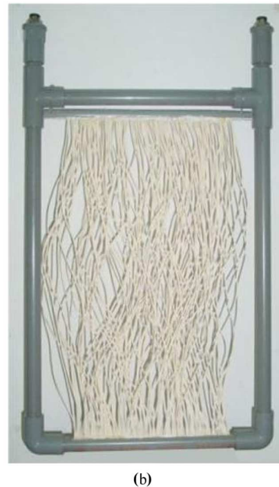
Fig. 1. (a) Overall schematic diagram and (b) membrane module of MCMFB system. (1) Raw wastewater. (2) Anaerobic influent. (3) Anaerobic effluent. (4) Permeate.
