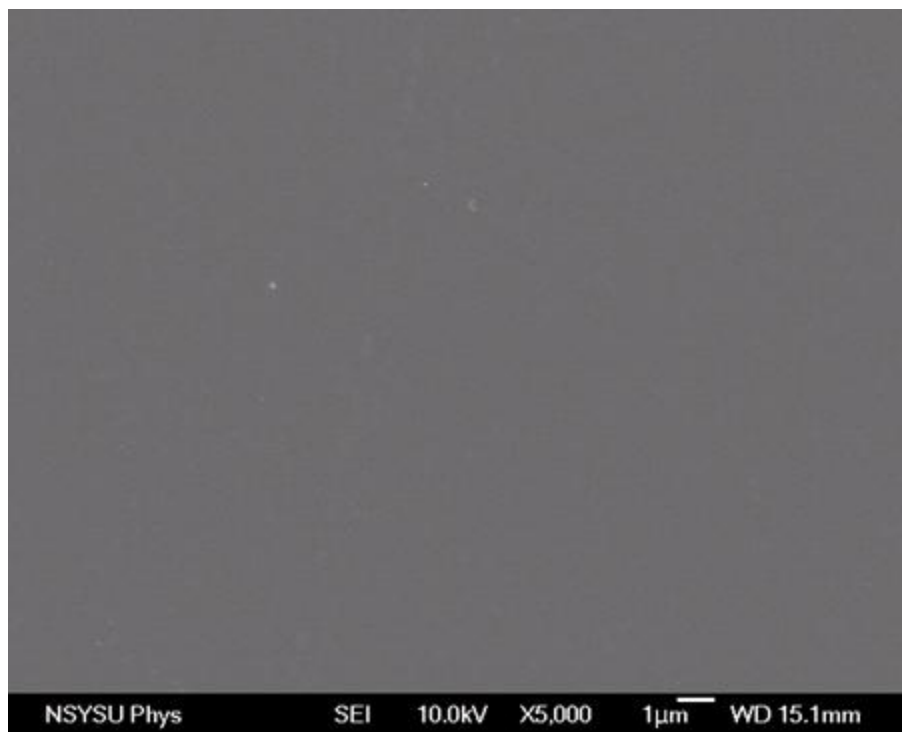
Fig5. 14 Plane view SEM image of freestanding GaN thick-film (李威儀教授實驗室)
