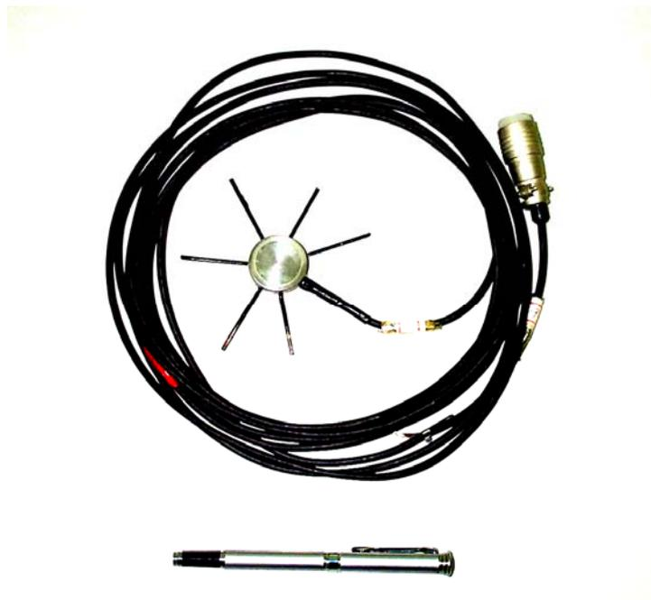
Fig. 7. Soil-pressure transducer (Kyowa BE-2KCM17) (after Chen, 2003)
