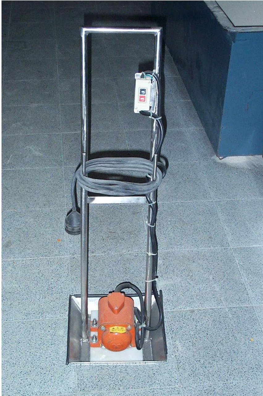
Fig. 8. Vibratory soil compactor (after Chen, 2003)
