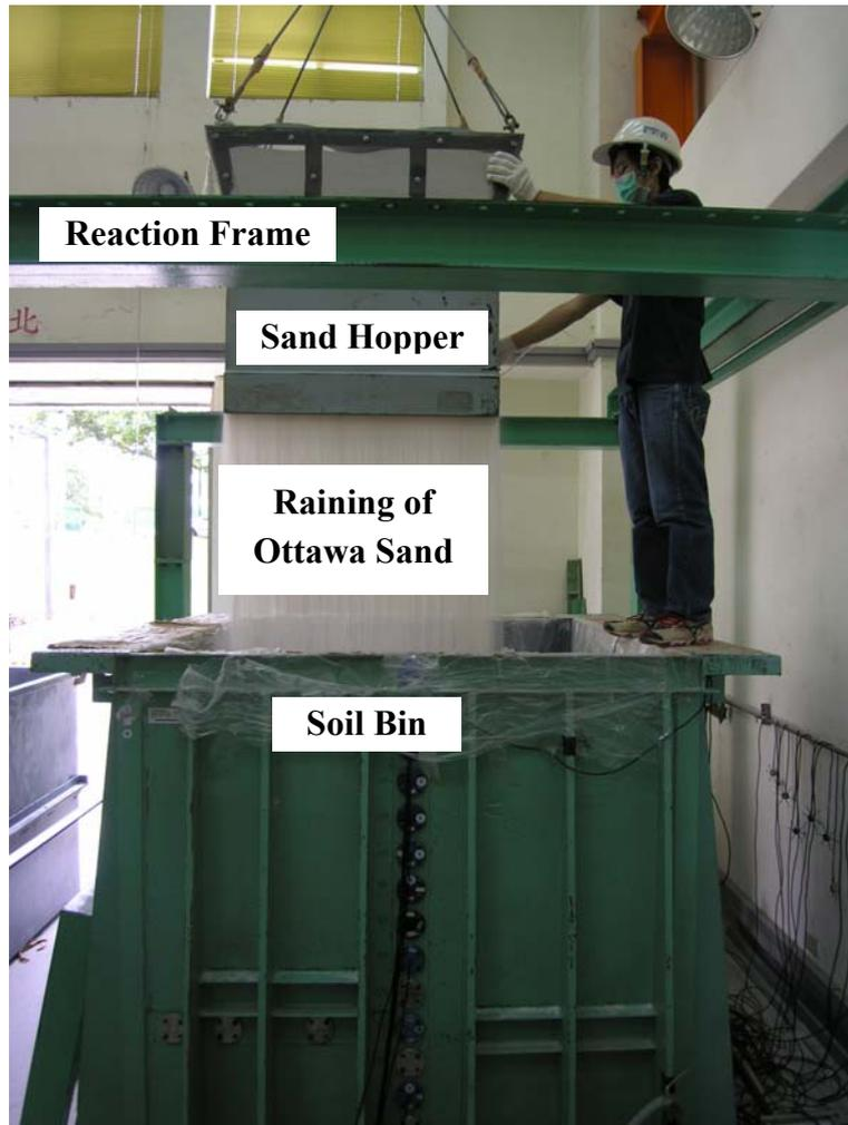
Fig. 10. Pluviation of the Ottawa sand into soil bin
