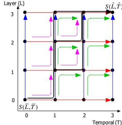
Figure 13: The Trellis Diagram of the bitstream meets the Weak Local Conditions
