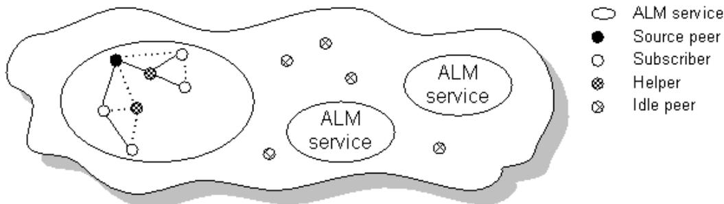
Figure 1 : Application Layer Multicast (ALM) System
