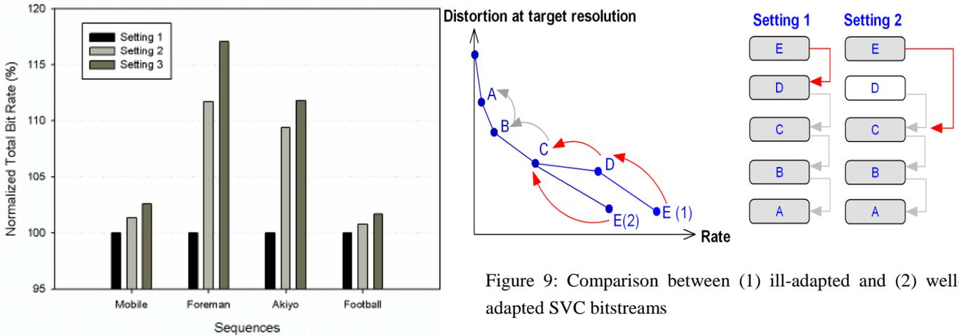
Figure 8: Comparison of coding efficiency based on different inter-layer dependencies. In our experiments, the optimal extraction paths for three viewing devices of CIF@30Hz, CIF@15Hz, and QCIF@30Hz formats were constructed by exhaustive search for the four test sequences: Mobile, Forman, Akiyo and Football.
