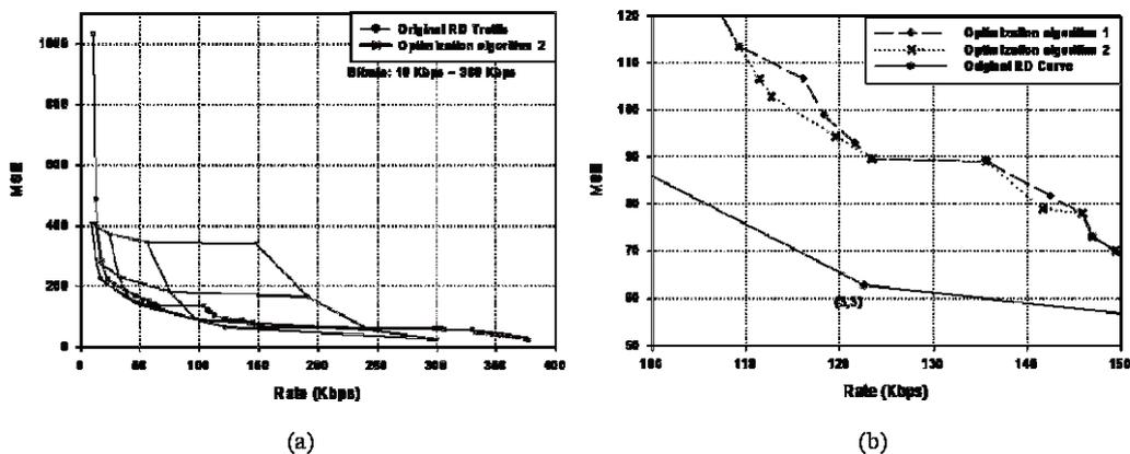
Figure 18: (a) Optimization Algorithm 2 RD Curve of optimal policies. (b) Compare Algorithm 1 to Algorithm 2 Min MSE at Different Bit Rate
