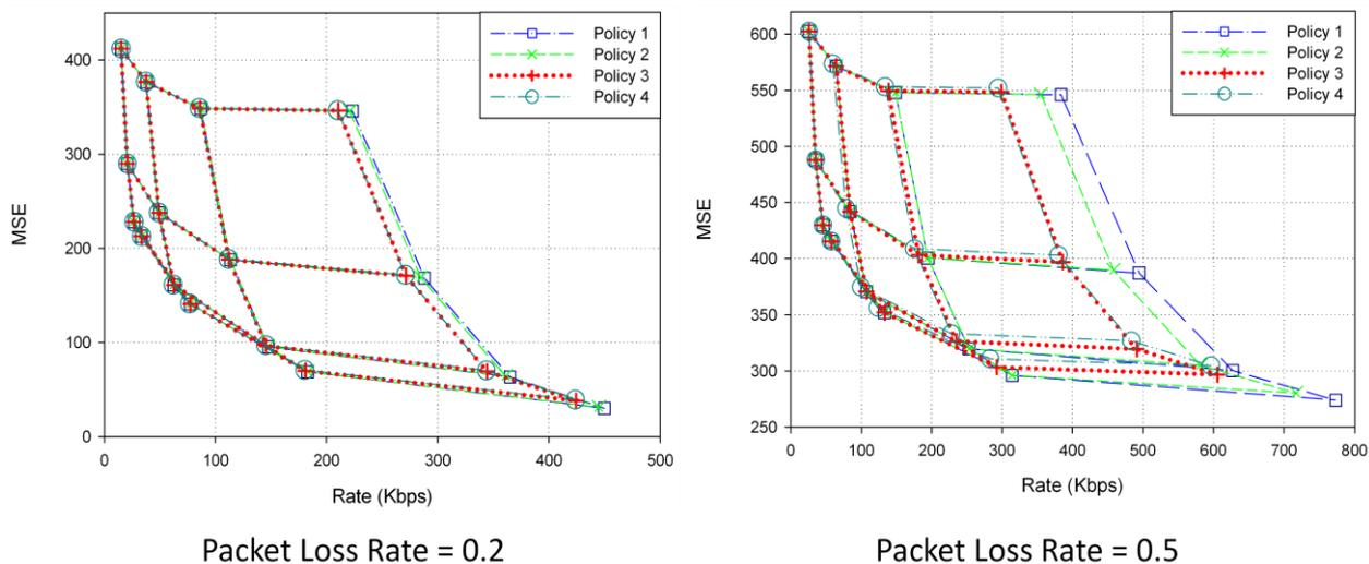
Figure 17: Different Policies, Different Packet Loss Rate in Receiver-driven Aggressive Retransmission
