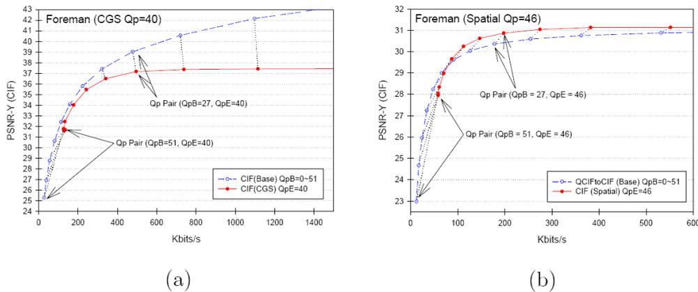
Figure 5: R-D performance of (a) CGS and (b) spatially scalable bitstreams with different  $Qp$  values
