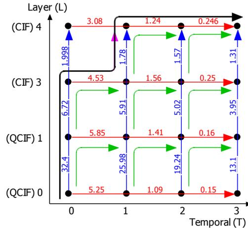
Figure 11: Corresponding Trellis Diagram of R-D Mesh in Figure 10
