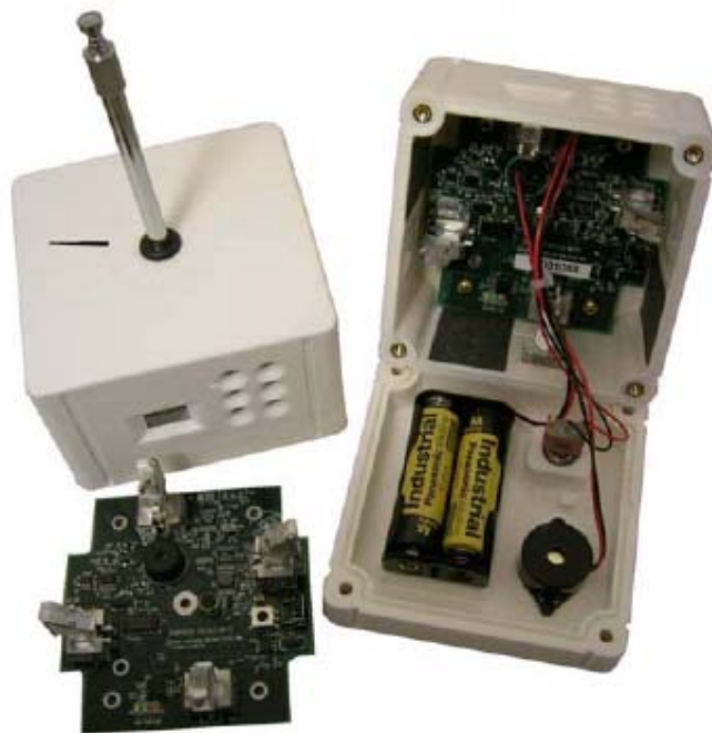
圖 2 ExScal hardware design
