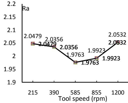
Figure 8 Simulation done by neural network w.r.t. tool speed (Ra in  $\mu\text{m}$ )
