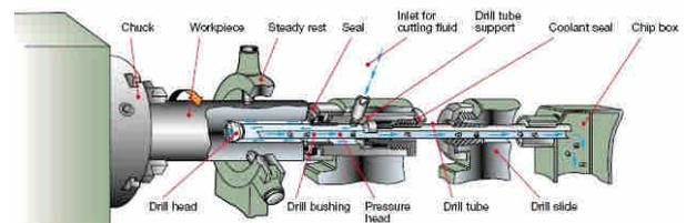
Figure 1 BTA Deep hole drilling process [4]
