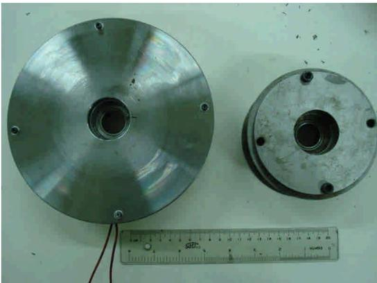
Figure 2 The designed magnetorheological fluid damper
