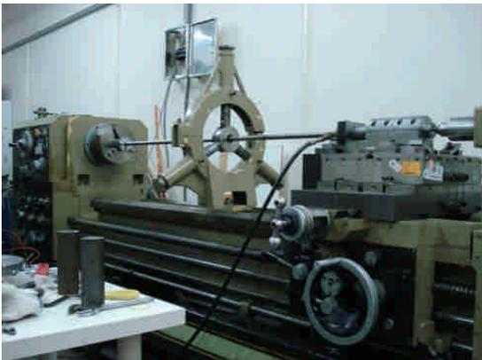
Figure 3 The testing machine for the new deep hole drilling process
