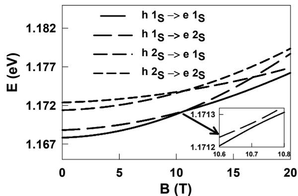
Fig. 3. Lowest transition energies in the double dot molecule as functions of magnetic field  $B||z$ . Inset: the anticrossing region.
