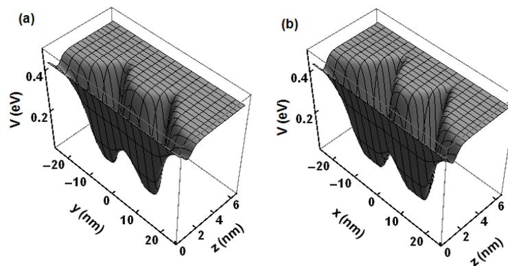
Fig. 10. Two projections of the confinement potential on (a)  $(0,y,z)$  and (b)  $(x,0,z)$  planes
