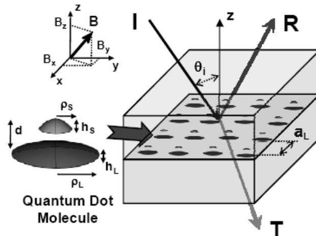
Fig. 2. Schematic of the magneto-optics of a layer of embedded semiconductor quantum dot molecules.
