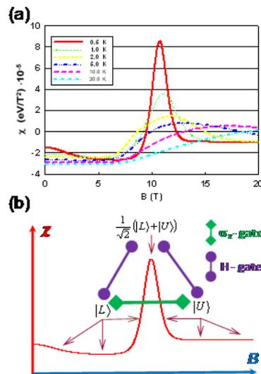
Fig. 7. Schematic of the quantum gate's realization in the asymmetrical quantum dot molecule: (a) magnetic susceptibility of the single electron asymmetrical double dot molecule at different temperatures; (b) quantum gate's control.
