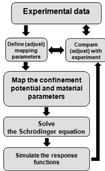
Fig. 8. Flow diagram of the mapping procedure.
