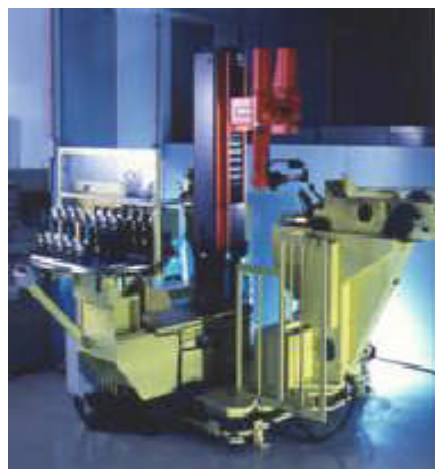
圖 5-11 Automated aerofoil restoration
