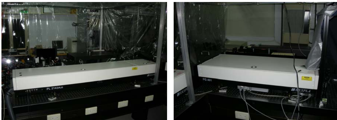
Fig. 2. Pictures of the EKSPLA laser system at IAMS. Left: picosecond Nd:YAG laser. Right: OPG/DFG part, which generates mid-IR light in the range of 2.3–18 \mu\text{m} ( 600\text{--}4000\text{ cm}^{-1} ).
