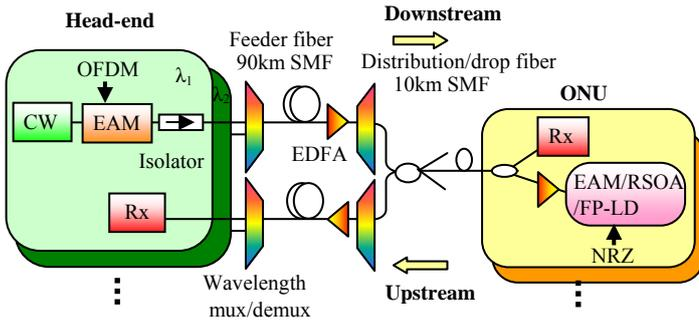
Fig. 6. Experimental setup of signal remodulation DWDM-PON. EAM: electro-absorption modulator, SMF: single mode fiber, EDFA: erbium-doped fiber amplifier, RSOA: reflective semiconductor optical amplifier, FP-LD: Fabry-Perot laser diode.
