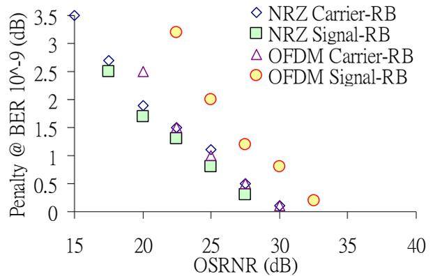
Fig. 3. RB noise performance at OFDM-QAM when compared with conventional NRZ formats.
