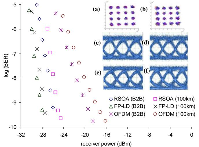
Fig. 8. BER measurements of different signals. Insets: constellation diagrams of OFDM signal at ER = 3.7 dB at (a) B2B, (b) 100km, output remodulated NRZ eye diagrams of FP-LD at (c) B2B, (d) 100km; and RSOA at (e) B2B, (f) 100km, when downstream OFDM at ER = 3.7 dB.
