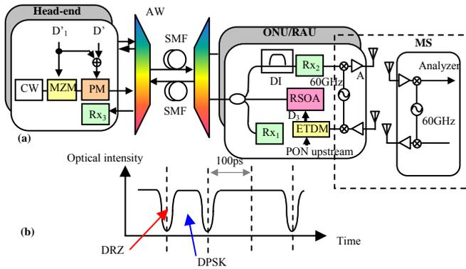
Fig. 2.1(a) Architecture of the wired/wireless access network. MZM: Mach-Zehnder modulator, PM: phase modulator, SMF: single mode fiber, AWG: arrayed waveguide grating, DI: delayed interferometer, A: RF amplifier, RAU: remote antenna unit, MS: mobile station, ETDM: electrical time division multiplexer. (b) Schematic time trace of the downstream signal carrying DRZ and DPSK.
