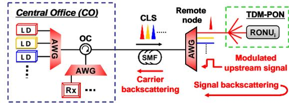
Fig. 1.1 RB contributions in a carrier distributed hybrid WDM-TDM PON architecture with RONU.
