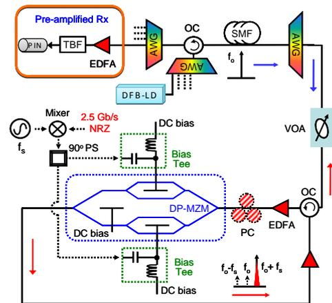
Fig. 1.2. Proposed carrier distributed PON using dual parallel-MZM (DP-MZM) as RONU. EDFA: erbium doped fiber amplifier, TBF: tuneable bandpass filter, VOA: variable optical attenuator, OC: optical circulator, PC: polarization controller, PS: phase shifter, 90° PS: 90° hybrid power splitter.
