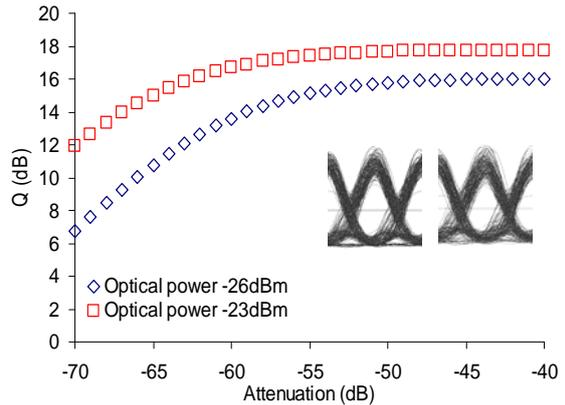
Fig. 2.3: Simulated Q (dB) of the down-converted BPSK signal at the MS under different attenuations between the RAU and the MS. Inset: simulated eyes of demodulated BPSK at MS when (a) Q=17.5dB (optical power at -23dBm) and (b) Q=16dB (optical power at -26 dBm).
