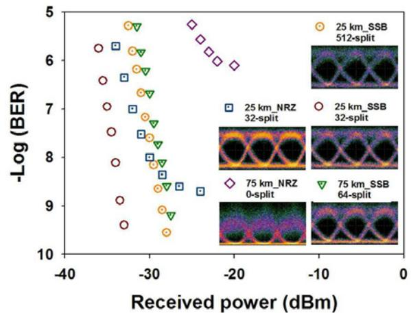
Fig. 1.4. BER performances of uplink SSB-NRZ (case 1) and conventional NRZ (case 2) signals with different split ratio in the transmission link. Insets show the corresponding eye diagrams.
