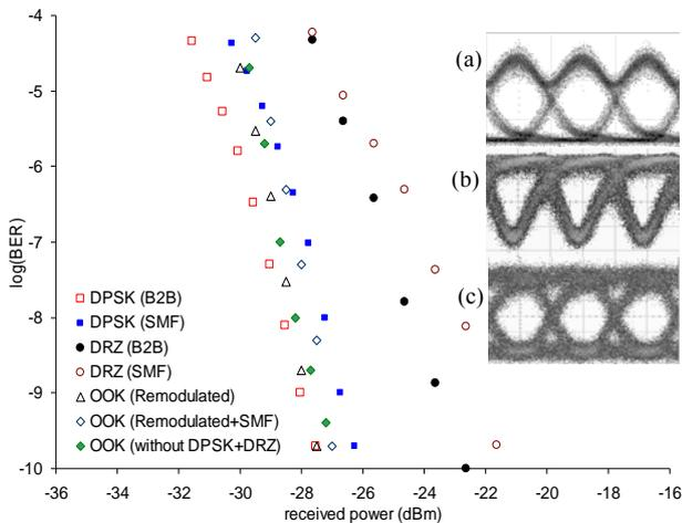
Fig. 2.2. BER measurements. Inset: eyes of (a) 10Gb/s demodulated DPSK (at Rx<sub>2</sub>), (b) 10Gb/s DRZ (at Rx<sub>1</sub>), and (c) remodulated 2.5Gb/s OOK (at Rx<sub>3</sub>) after transmission.
