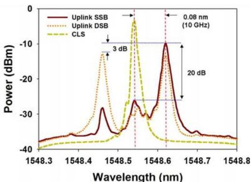
Fig. 1.3. Measured optical spectra. Solid line: SSB-CS uplink signal. Dotted line: DSB-CS uplink signal. Dashed line: centralized light source (CLS).
