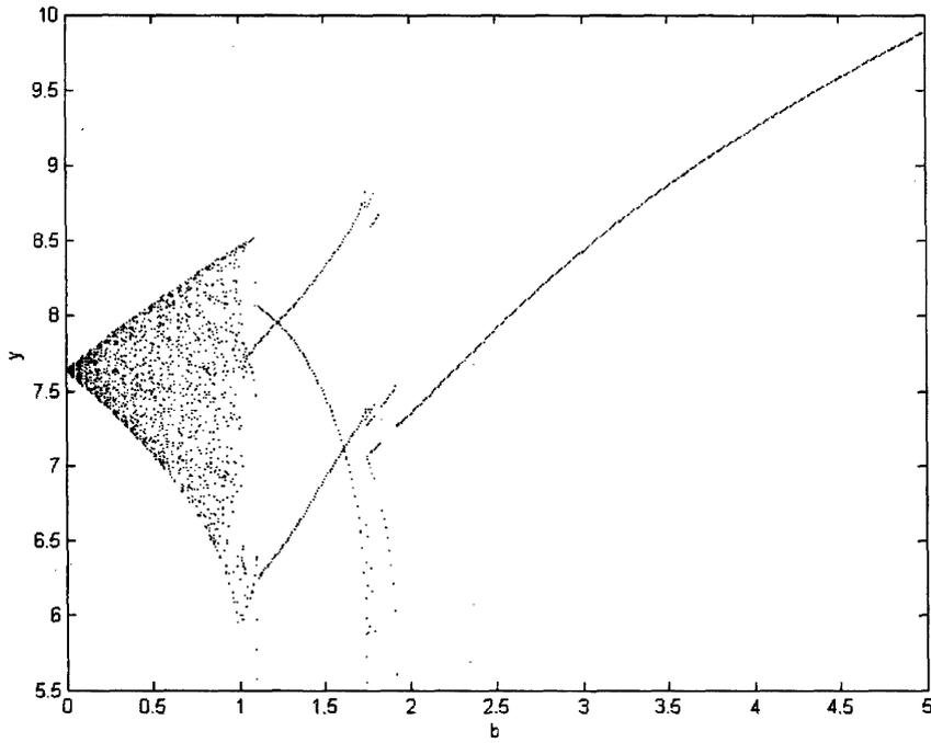
Fig. 1. The bifurcation diagram for  $\alpha = \beta = 1$ .
