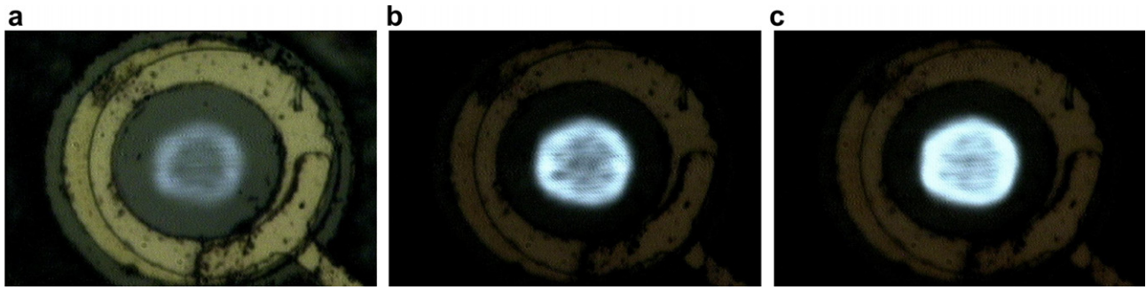
Fig. 7. Near-field images of InGaAs SML QD VCSEL without PhC at (a) 3 mA, (b) 7 mA, and (c) 10 mA.
