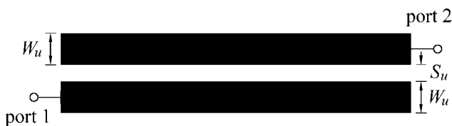
Fig. 1 Uniform microstrip coupled stage as a two-port network
