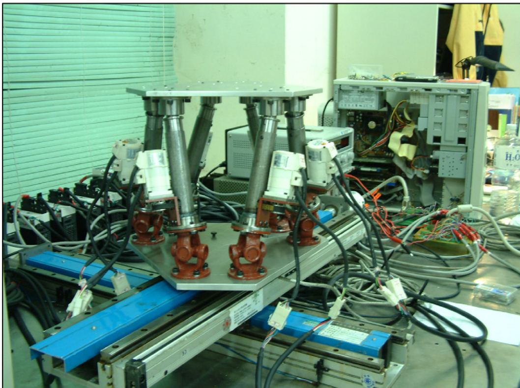
Fig. 6. Multi-axis machine tool with parallel upper structure and XY-base.
