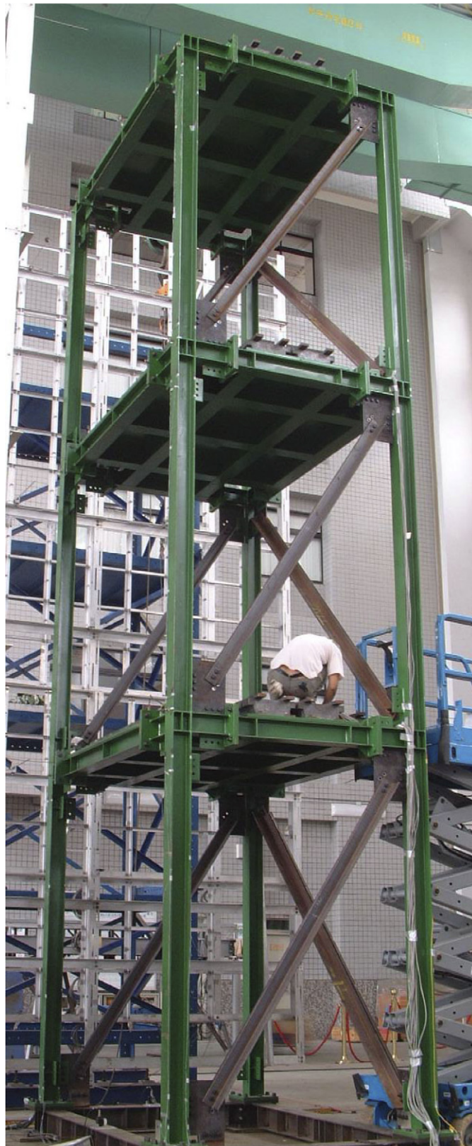
Fig. 8. Photo of a three-story non-symmetric steel frame.
