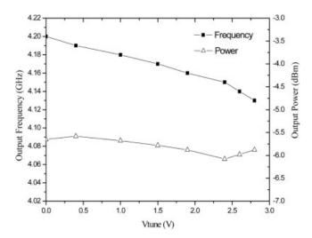
**Figure 3** Output power and frequency as a function of the tuning voltage for the superharmonic-coupled SiGe HBT QVCO
