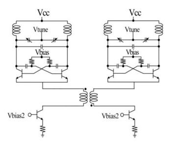
Figure 1 Schematic of the superharmonic coupled SiGe HBT QVCO
