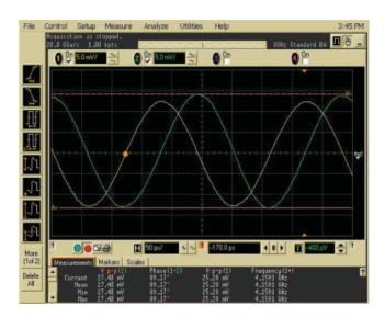
**Figure 5** Time-domain I/Q channel waveforms of the superharmoniccoupled SiGe HBT QVCO.[Color figure can be viewed in the online issue, which is available at www.interscience.wiley.com]
