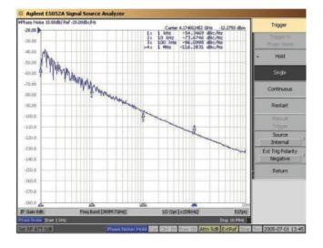
**Figure 4** Phase noise spectrum of the superharmonic-coupled SiGe HBT QVCO. The phase noise is -116 dBc/Hz at 1 MHz offset frequency when the oscillation frequency is 4.17 GHz. [Color figure can be viewed in the online issue, which is available at www.interscience.wiley.com]
