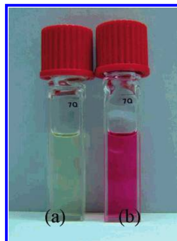
FIGURE 7. Colors of (a) 6 (10 \mu\text{M} ) in a methanol-chloroform (v/v = 1/399) cosolvent at 25 ^\circ\text{C} and (b) 6 after adding 5 equiv of Hg(ClO _4 ) _2 .
