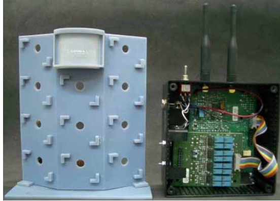
Fig. 2. A sensor module (including a PIR detector, a Fresnel lens array, Texas Instrument micro-controller (MSP430149) and RF transceiver (TRF6901) module)
