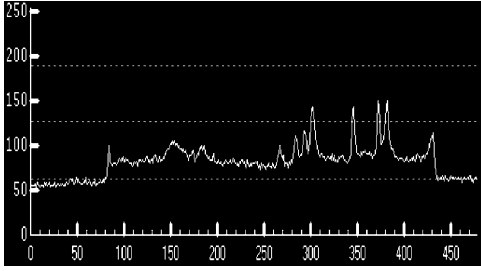
Fig. 4. Intensity profile of a vertical scan line passing through the middle of a lane.
