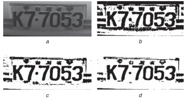
Fig. 2 Licence plate processed by BAT, OAT and MAT
