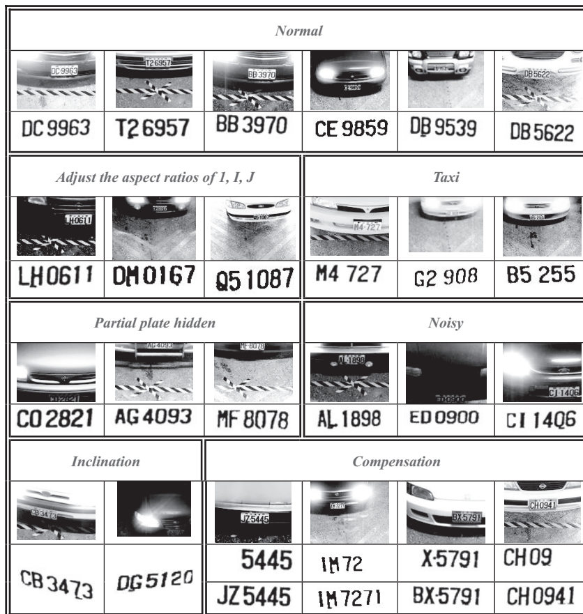
Fig. 8 Some of the images from which the proposed system successfully extracted characters
