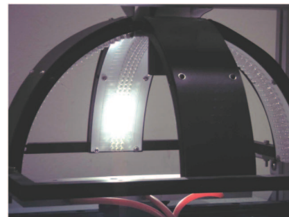
Fig. 13. (Color online) (a) Side view of the proposed structured lighting system. For clarity, only the east and west strips of LED arrays and associated soft PCBs are depicted. (b) 3D illustration of the structured lighting system. (c) Photograph of the prototype of the proposed structured LED lighting system.
