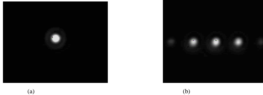
Fig. 8. Diffraction patterns (a) before and (b) after applying voltage to the actuator.
