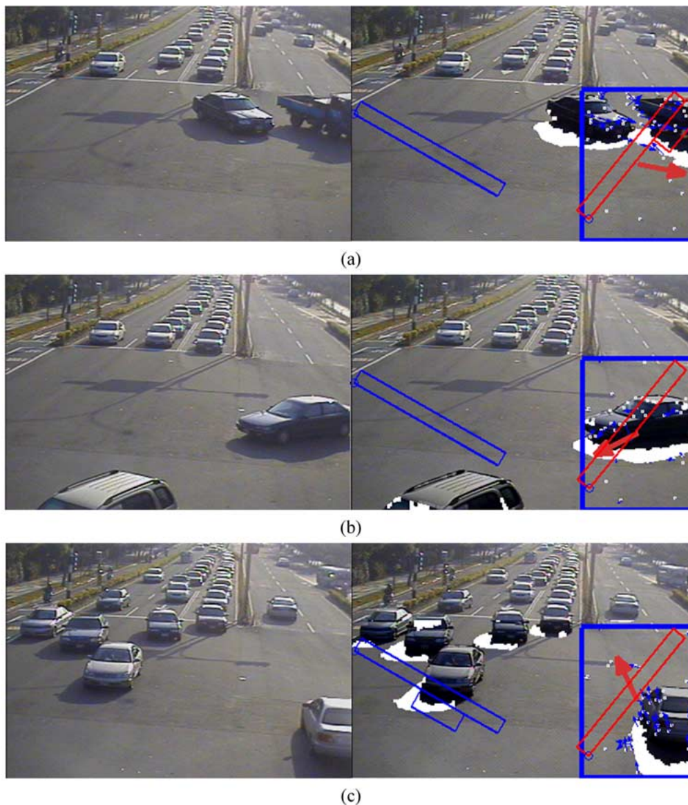
Fig. 8. Experimental results of turn ratio estimation with shadow suppression at an intersection. Three types of driving direction of vehicles are distinguished: (a) moving right, (b) moving left, (c) moving straight ahead.
