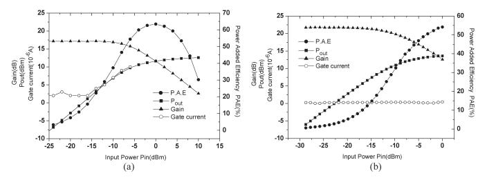
Fig. 5. (a) Power performance and gate leakage current of the  $0.7 \times 240$ - $\mu$ m E-mode PHEMT before gate sinking. (b) Power performance and gate leakage current of the  $0.7 \times 240$ - $\mu$ m E-mode PHEMT after gate sinking.
