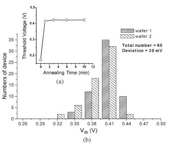
Fig. 4. (a) Threshold voltage of the Pt/Ti/Pt/Au E-mode PHEMT versus annealing time when annealed at 325 °C. (b) Distribution of  $V_{\rm th}$  for the E-mode PHEMT across 4-in wafer for two different wafers.
