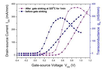
Fig. 3. Transconductance and the drain-source current versus  $V_{\rm GS}$  curves of the 0.7 × 240- $\mu$ m E-mode PHEMT at  $V_{\rm DS}$  = 2 V with 20-nm thick-Pt before and after gate sinking at 325 °C for 1 min.
