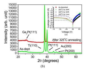
Fig. 2. (a) I-V characteristics of the diodes before and after annealing. (b) XRD spectra of the Pt/Ti/Pt/Au and InGaP/AlGaAs/InGaAs PHMET sample before and after annealing at 325 °C for 3 h. Main component: Ti, Pt, Au, Ga<sub>2</sub>Pt (JCPDS PDF 44-1288, 04-0802, 04-0784, 03-1007).
