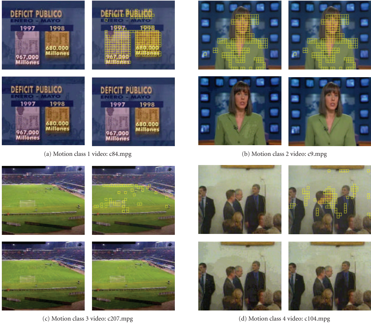
FIGURE 18: Comparison of visual quality. (1) The upper-left is original video. (2) The upper-right is information object result of video analyzer. (3) The bottom-left is the result video of normal uniform adaptation. (4) The bottom-right is the result video of our proposed adaptation.
