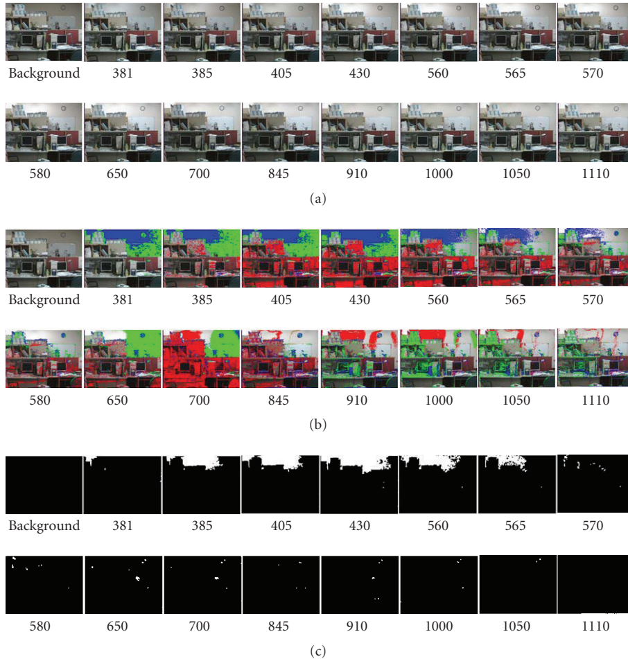
FIGURE 8: The results of global illumination changes with fluorescent lamps, the number below the picture is the index of frame, (a) original images, (b) the results of pixel classification, where red indicates the shadow, green indicates the highlight, and blue indicates the foreground, (c) the results of background subtraction with shadow removal using our proposed method, where dark indicates the background and white indicates the foreground.
