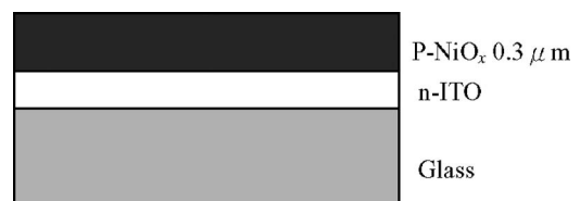
FIG. 1. A schematic structure of the NiO x /ITO/glass heterojunction diode. The sheet resistances of the ITO and NiO x are 70 and (6–18) × 10 6 Ω/□, respectively.
