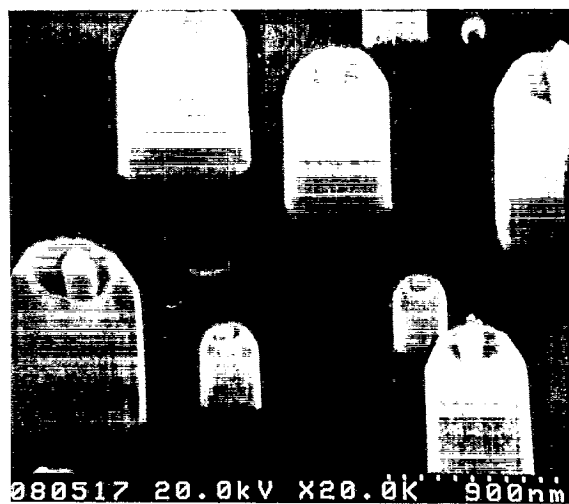
Fig. 4. The surface profile and surface morphology of the etched GaN: (a) etched profile of GaN etched at RF power 300 W, 40 mtorr, 20 sccm \text{BCl}_3/20 sccm \text{SF}_6 for 25 min and (b) 'candle like' residues on the etched area.
